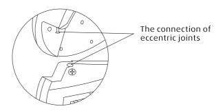
▶ The connection of armrest locks with backrest. Hold up the rear part of the armrest, push inward to let the gap of armrest lock aim at armrest spindle, then push the armrest to fasten them together.(Press downward the handle of the lock to unlock armrest and backrest)
